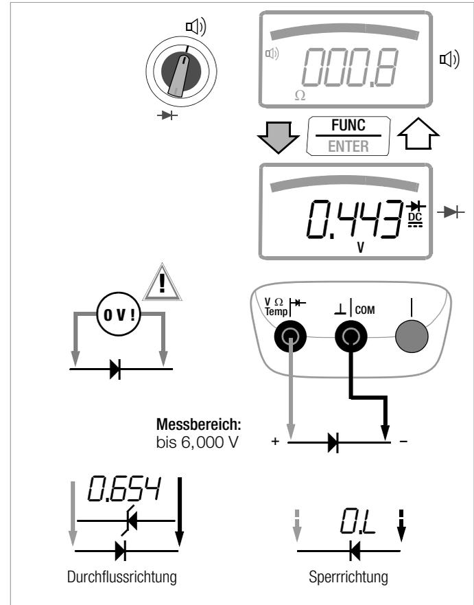
The diagram illustrates the procedure for diode testing. It shows a rotary switch being set to the diode symbol, followed by pressing the **FUNC | ENTER** button. The display then shows a reading of **0.443 V** with a diode symbol and a **DC** indicator. A circuit diagram shows the diode connected to the **V Ω Temp** and **COM** ports. The display shows **0.654** for forward current direction and **.OL** for reverse current direction. The text **Messbereich: bis 6,000 V** is also present.
